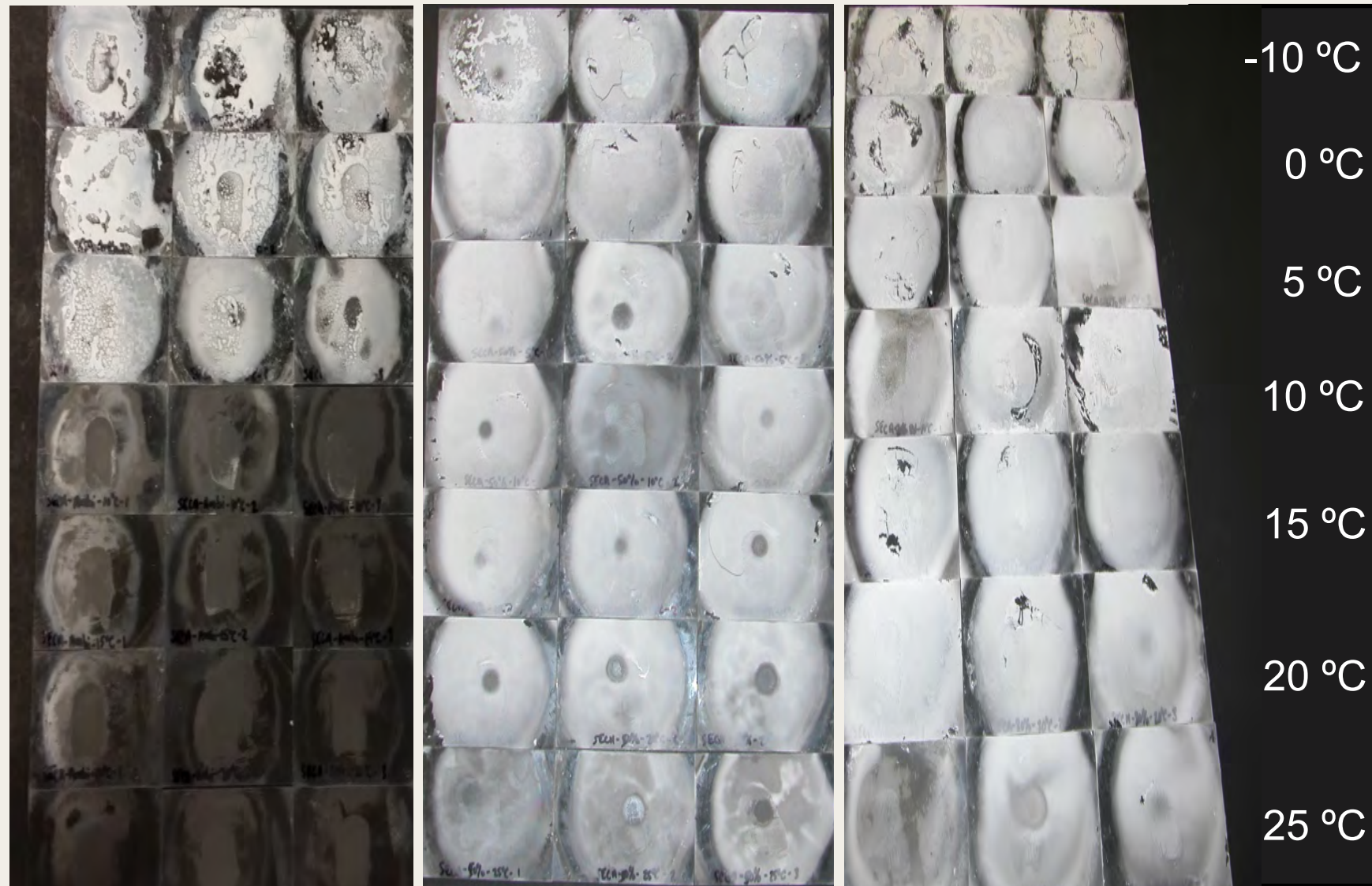
Figure 1: Photos of slides after fuming at surface temperatures from -10 to 25 °C at 50% (left) and 80% (right) relative humidity.
